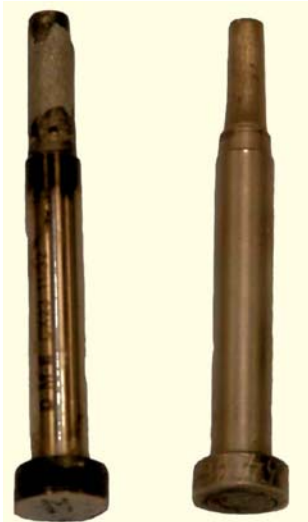
Untreated and treated H 13 tool steel die pins after 3,500 and 200,000 shots of aluminum, respectively.
