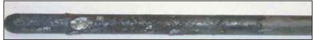
MIST-coated probe after 467 cycles. In dip tests in molten aluminum at a temperature of 760°C, life of z-MIST treated 1010 steel thermocouple sheaths reportedly had eight times longer service life than that of untreated sheaths.
