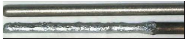
Thermocouple sheaths after exposure to molten aluminum; probe at bottom shows condition of untreated probe after 91 cycles.
